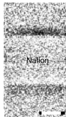
Fig. 5. Infrared radiation image of Nafion-117 in water. Nafion strip runs horizontally (central zone cropped for clarity). Scale: 1 mm between black dots. Darker areas indicate reduced radiation intensity. Interfacial regions, just beyond the edges of the Nafion strip, radiate appreciably less than more remote regions.
